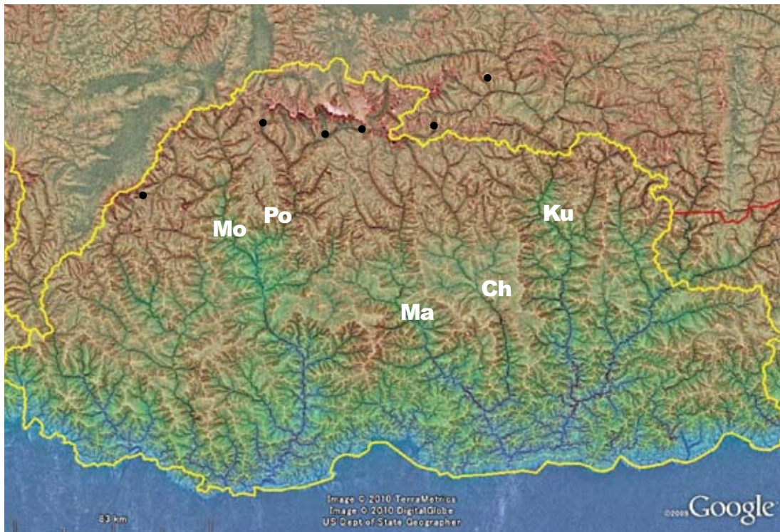
Fig. 1 Topographical map of Bhutan. The map was created by Mr. Tatsuro Chiba (Asia Air Survey Co., LTD.) on Google Earth using Red Relief Image Map method (RRIM, Chiba et al., 2008) with SRTM DEM. The map expresses regional difference in geomorphological condition, such as deep valley in the great Himalaya, dendritic valleys and erosion fronts in southern half of Bhutan. M: Mangde Chhu. C: Chamkhar Chhu. Solid circle: Outburst glacier lakes after the little ice age termination (see Table. 1).
