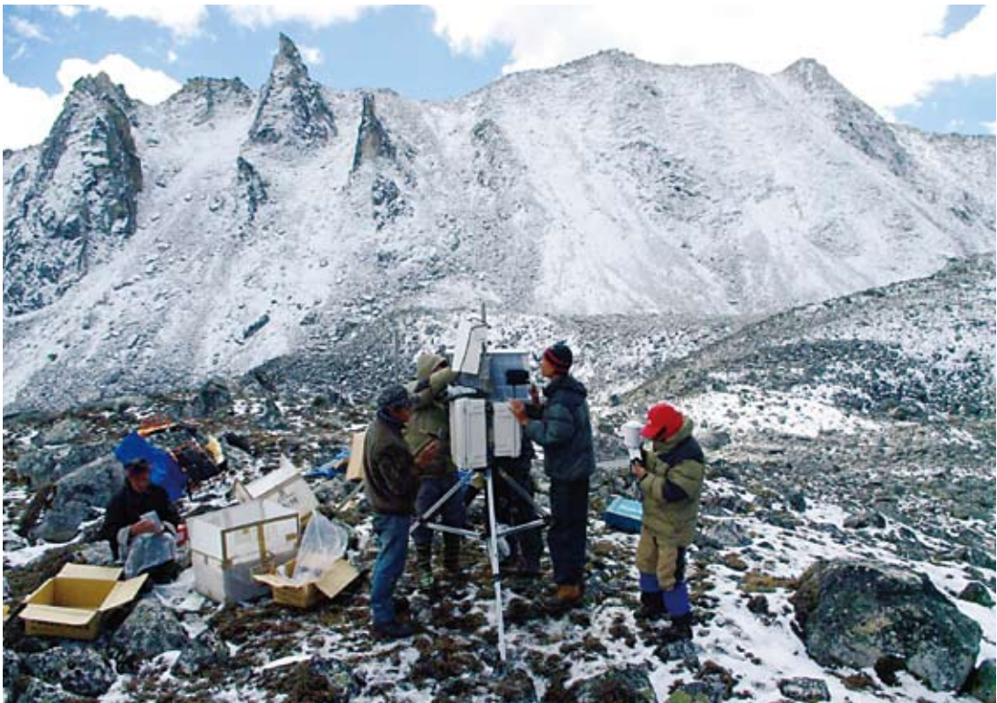
Photo. 5 Installation work of the automatic weather station on the moraine in September 2009 . The station had been keep stable condition except for the theft of tensioning wires by the local people. Lightly snow dusted ridge in the back in the photo is 5,500 ~ 5,400 m peaks (27.965° N, 90.335° E).
